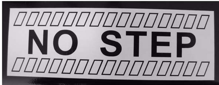
Figure 2-1. This warning label is on the top of both trailer fenders. Do not step on the trailer fender to reach any part of the equipment. (Part no. 59-084-00)
