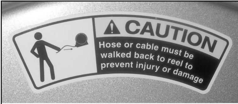
Figure 2-4. This label is on the hydraulic hose reel. When retracting the hose, walk it back to the reel. Do not let the hose snap back into the reel. (Contact the manufacturer, Cox Reels, for replacement labels.)
