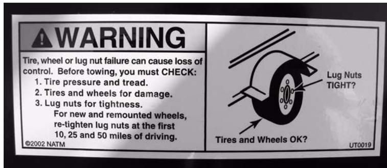
Figure 2-3. This warning label is on the back of both trailer fenders. Prior to each use of the trailer, check tire condition and lug nut tightness. (Part no. 77-160-15)
