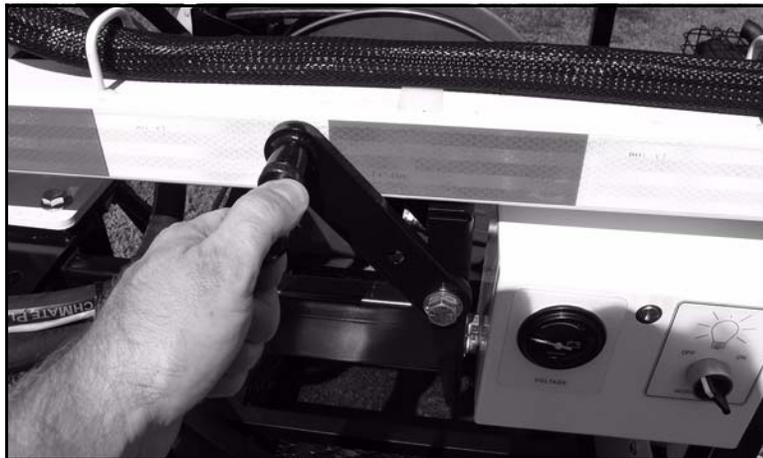
*Figure 4-7. Move the latch down while pulling the knob out.*
