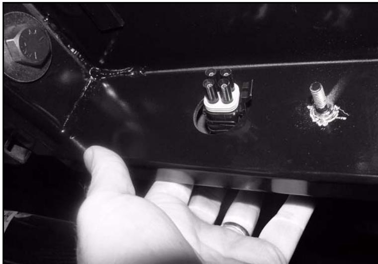
*Figure 3-5. Route tongue connectors through frame.*
