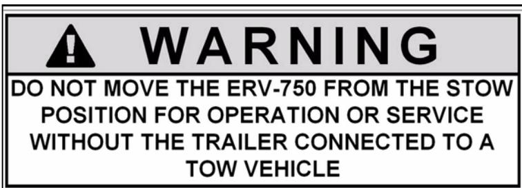
Figure 2-6. This warning label is on the ERV head. Before moving the ERV from the stow position, ensure that the trailer is connected to a tow vehicle (Part no. 79-020-00-01.)
