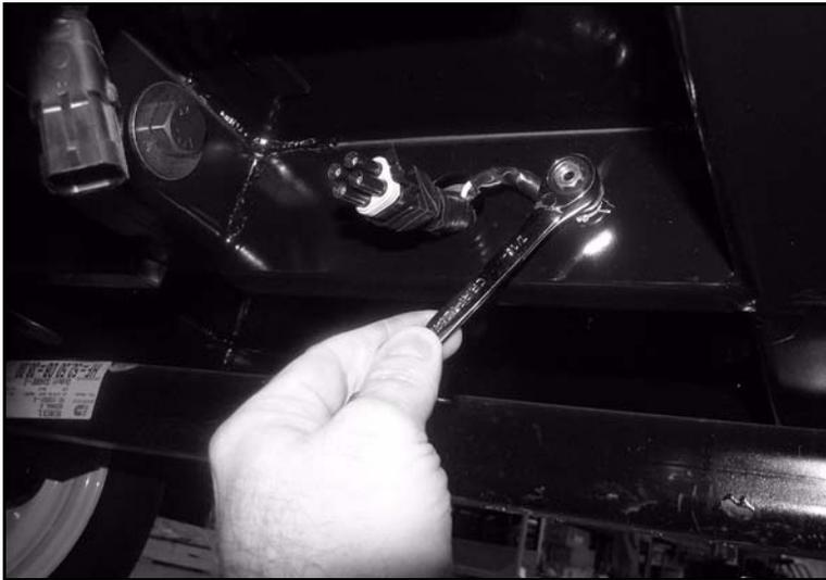
*Figure 3-6. Attach ground wire to stud.*
