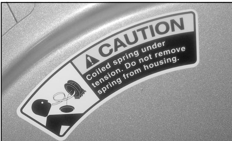
Figure 2-5. This caution label is on the hydraulic hose reel. Do not disassemble the spring from the reel.
