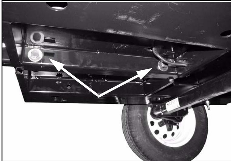
*Figure 3-4. Tighten nuts to secure tongue to trailer.*
