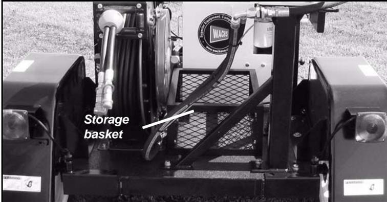
*Figure 3-15. The storage basket is mounted at the rear of the trailer.*
