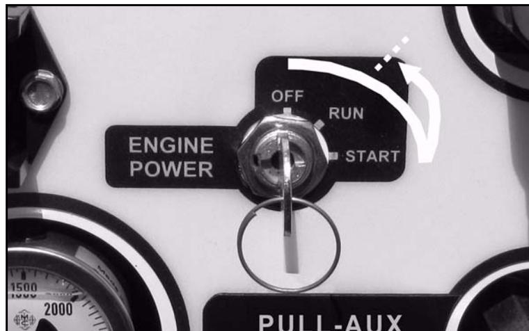
Figure 4-2. Turn the key to **START**, then release to **RUN** when the engine starts.
