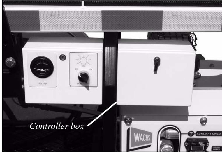
*Figure 4-11. The light bar controller is inside a box on the right side of the trailer.*
